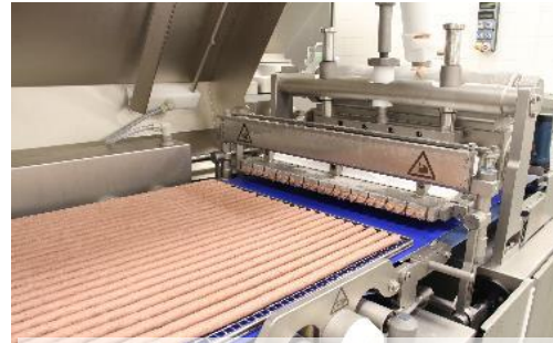
Molding with dies/pipes
