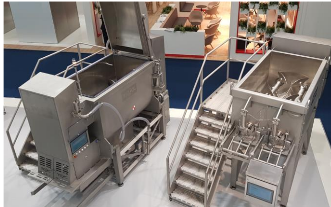
IM, IMP, IMS series: conventional mixers from 500 – 6.000 Liters
