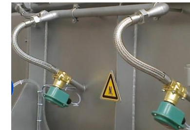
cryogenic cooling by direct injection
